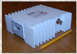
This small and light weight 2W L-To C-Band Block Up Converter is designed to be mounted on the feed horn. High power efficiency resulting in low current (<= 1.5 amps) consumption allows user to pass DC supply voltage via IF cable. The unit is ideal for network and point to point, data distribution, portable and emergency applications.
