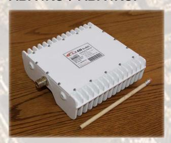
This small and light weight 4W L-To Ku-Band Block Up Converter is designed to be mounted on the feed horn. High power efficiency resulting in low current (<=2 amps) consumption allows user to pass DC supply voltage via IF cable. The unit is ideal for network and point to point, data distribution, portable and emergency applications.
