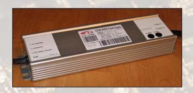
This slim and light outdoor power supply is suitable for various VSAT applications, which require 24 VDC output and 90-264 VAC input. The unit is equipped with short circuit, overload, over voltage, over temperature protection and certainly is in compliance to worldwide safety regulations.
