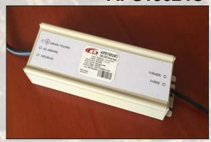
This slim and light outdoor power supply is suitable for various VSAT applications, which require 24 VDC output and 90-295 VAC input. The unit is equipped with short circuit, overload, over voltage, over temperature protection and certainly is in compliance to worldwide safety regulations.
